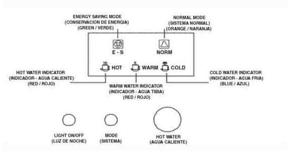
For operation of unit, please fill water and make sure water settles inside the water tank, and then switch on both hot and cold switches at back of unit.
